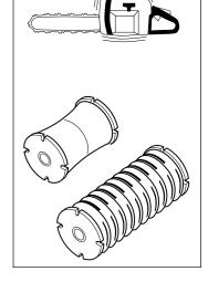
Make sure the vibration damping units are securely attached to the engine unit and handles.
